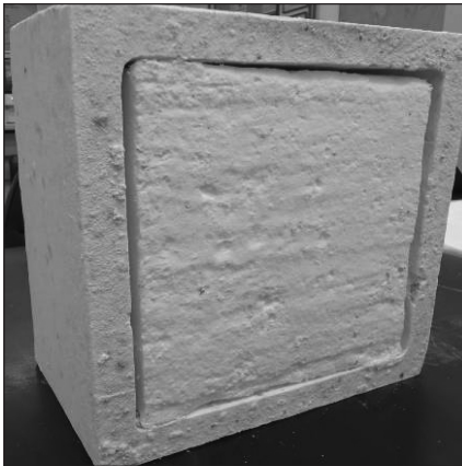
Module without Silplate Mass 1500 Shrinkage in excess of 3%
